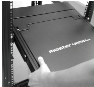
2. Slide the LCD KVM Switch / LCD Console onto the rails and secure it to the rack.
